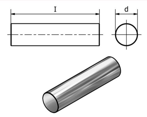
$\begin{array}{ll} \text{d1} & = 5 \\ \text{I} & = 20 \\ \text{Nominal adhesive forces} = 2.3 \\ \text{Weight in g} & = 450 \\ \end{array}$
